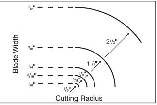
Figure 48. Recommended cutting radius per blade width.
